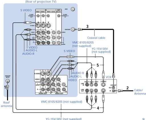
Connecting a VCR and projection TV to a cable box
